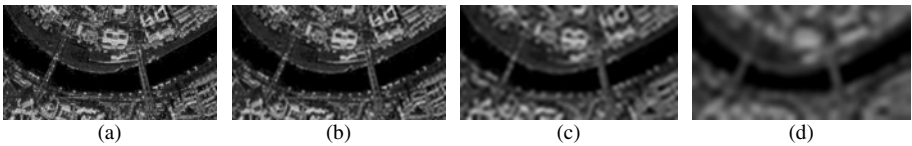
Fig. 2. SAR image and its NSP decomposition: (a) the original SAR image; subband of (b) stage1; (c) stage 2; (d) stage 3
